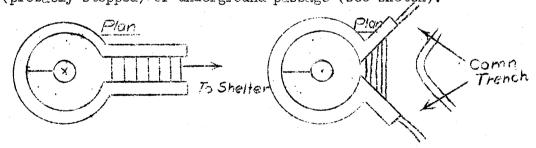
b. Dug in MG posts are known, but probably exist only as temporary positions till fortified posts are available, or in lightly defended areas. They consist of a semi-circular pit of 7 ft diameters and about 4 ft 6 in deep; the spoil is heaped in front in a semi-circle forming a parapet about 10 in high. (see sketch).
