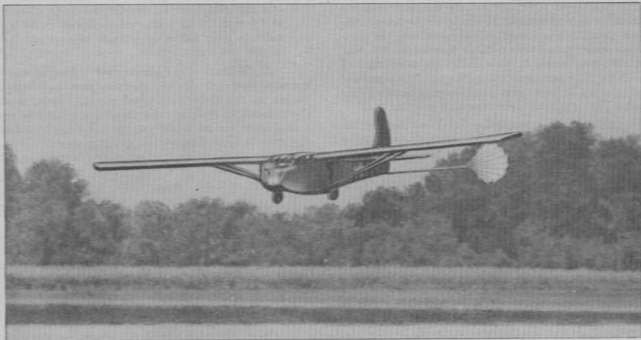
Figure 5—Showing Use of Deceleration Parachute
