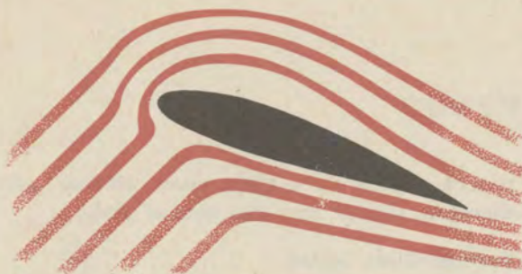
1. Wing close to stalling angle of attack
