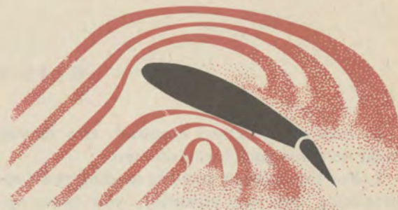
2. Lowering of aileron has same effect as increasing angle of attack, causing aileron stall. Wing drops instead of rising
