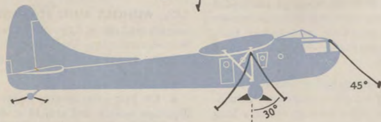
Figure 19. Tie-down methods CG-4A.
