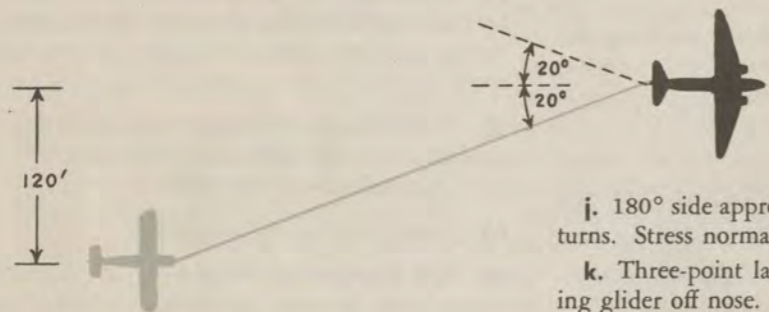
Figure 9. Angular limits for towing.
